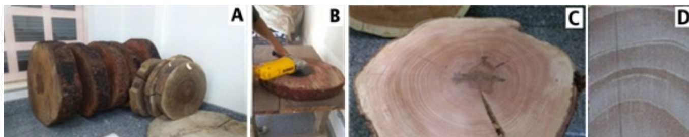
Figure 2. Preparation of samples for growth ring delimitation. Drying of the discs (A); Polishing of the discs (B); and Visible growth rings (C and D).
