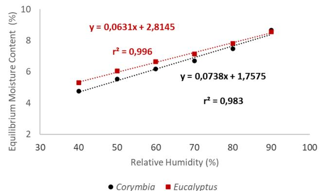
**Figure 2.** Observed difference in charcoal equilibrium moisture as a function of relative humidity.
